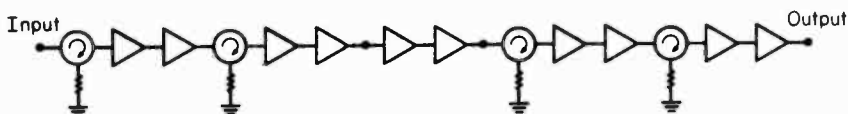
Fig. 5—Block diagram of final design of limiting amplifier. The frequency range is 8 to 11 GHz; the input power range is from -50 to 0 dBm; and the output power > +9 dBm.
